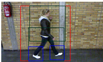
Fig. 2 Bounding boxes for human body parts: right and left feet (small blue boxes at the bottom), upper and lower body (green boxes in the middle) and full body (big red box)
